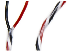
Nordost wyrewizard used as the internal cable for the four woofers
